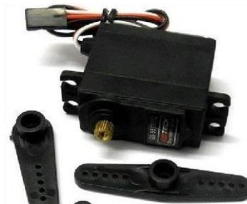
Figura 3 Servomotor MG995.
