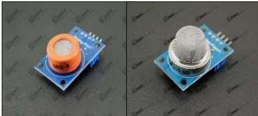
Figura 4. Sensor MQ-3 y sensor MQ-135
